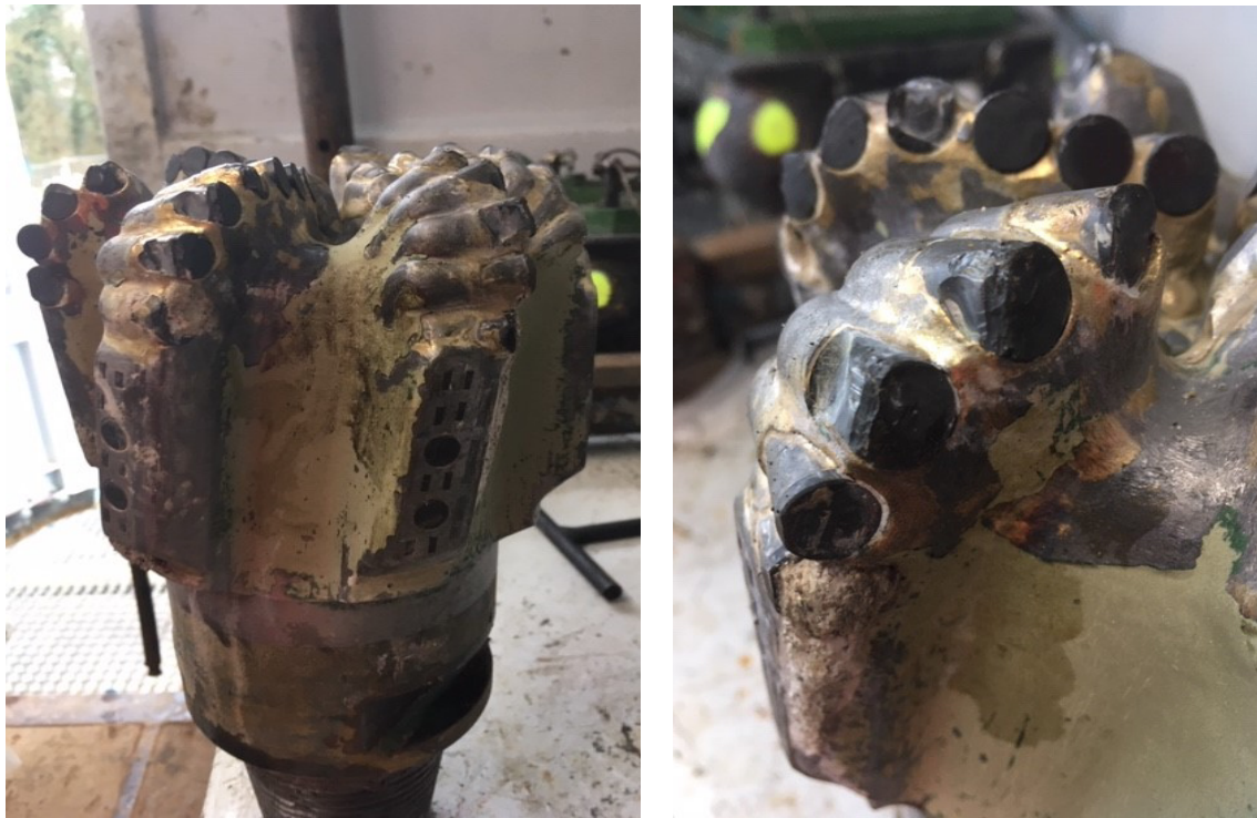
Fig. 3-4: 6½" PDC bit after POOH
