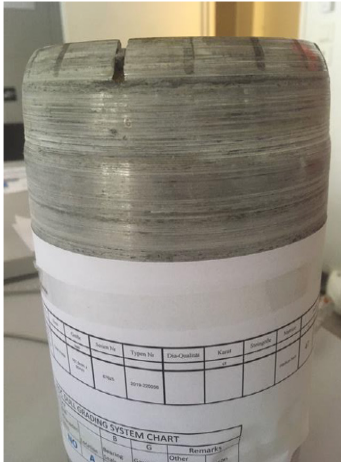
Fig. 3-11: Impregnated core bit fully destroyed without any matrix
