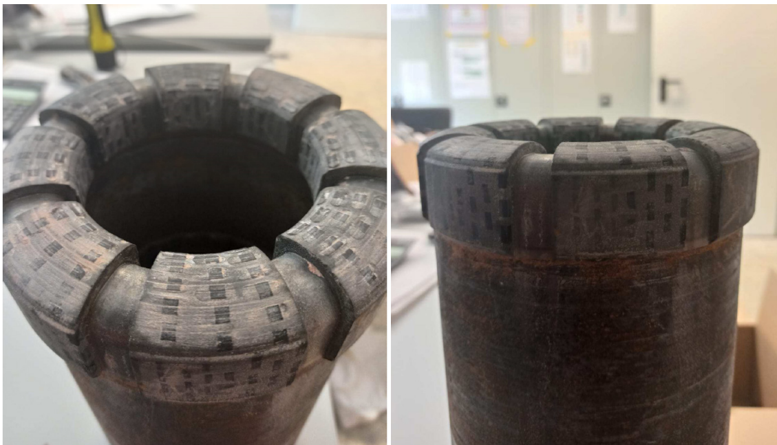
Fig. 3-12: Synset core bit after pulling out of hole at a depth of 1'054 m MD
