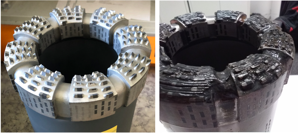
Fig. 3-7: Synset core bit before RIH (left) and after POOH (right) from a depth of 655 m MD
