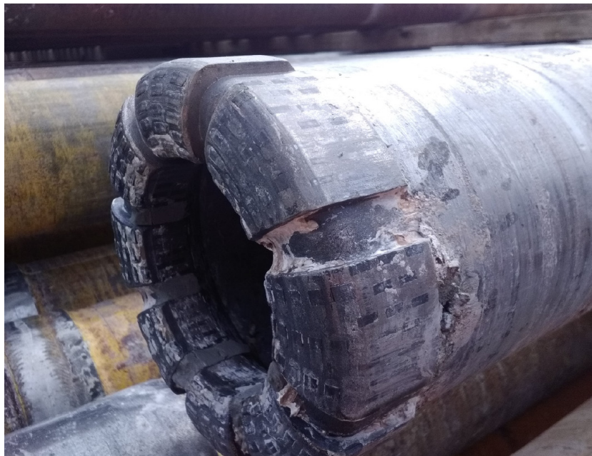
Fig. 3-8: Synset core bit after POOH from the depth of 796 m MD
