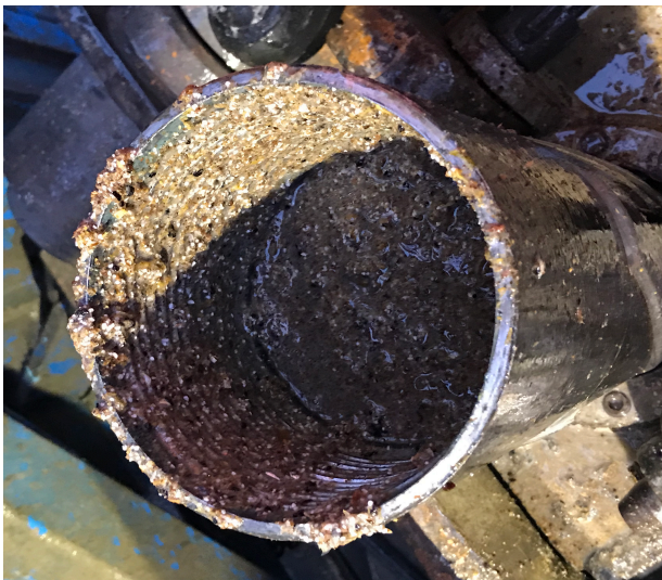
Fig. 3-10: Equipment contaminated and plugged with LCM material
