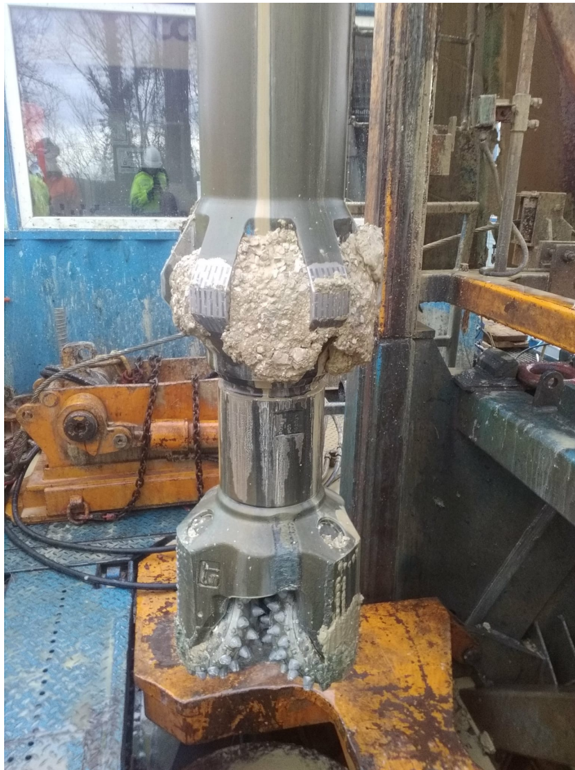
Fig. 3-3: 17½" tricone bit and 9⅝" mud motor after POOH
