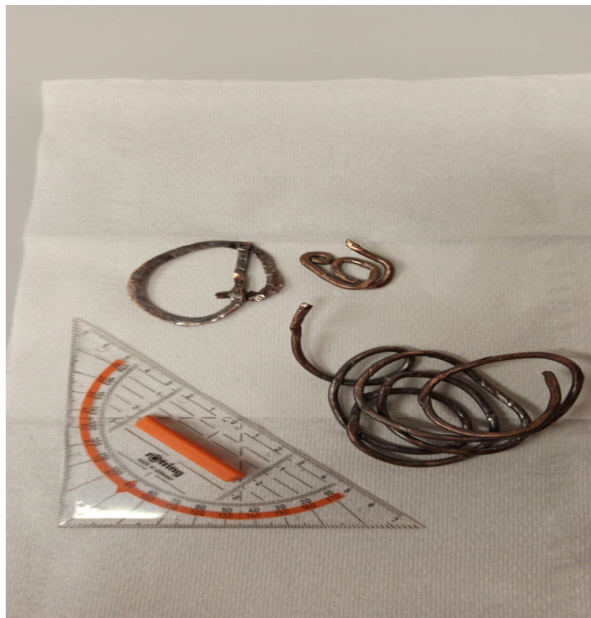
Fig. 3-5: Junk in hole recovered from 463 m MD
