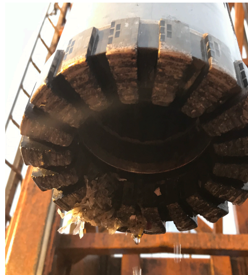
Fig. 3-10: Equipment contaminated and plugged with LCM material
