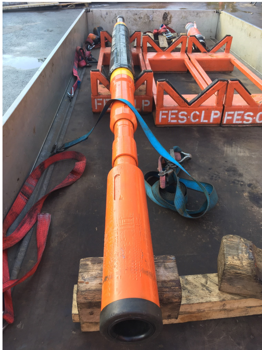
Fig. 3-13: 5½" open hole bridge plug with straight pull release
