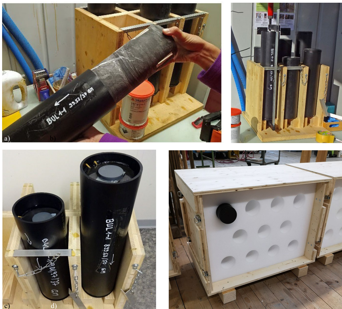
Fig. 3-1: Sampling and storage workflow of GM cores
