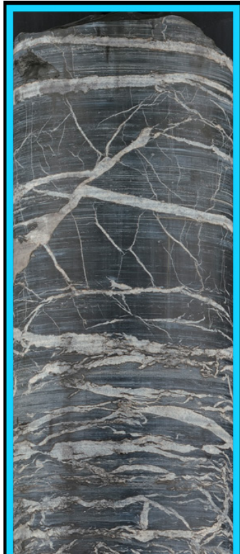
Fig. 4.3-3: Core photograph of heterogeneous sample 659.95 from the Bänkerjoch Formation Width of photograph is 10 cm.
