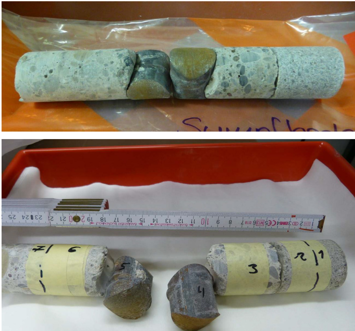
Fig. 2-1: Drill core extracted from the containment building of KKB Unit 2 Pisano (2018)
