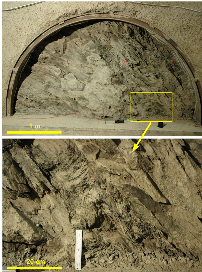
Fig. 5-1: The Main Fault in the Gallery 98 of the Mont Terri underground laboratory Upper picture shows the whole fault in the right half of the window. Detail in the lower picture illustrates a zone with a high degree of shear deformation, including drag folding.
