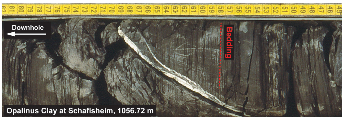
Fig. 3-20: Calcite III as infill of a slickensided fracture crosscutting bedding.
