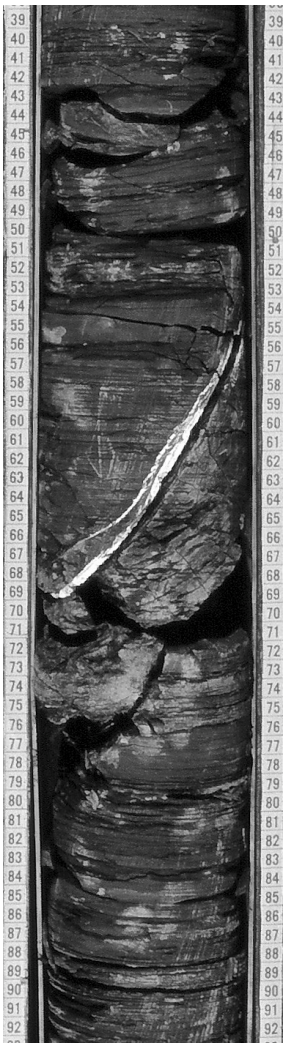
Fig. 5-5: Slickensided fracture sealed with vein calcite at 1'056.66 m in the Schafisheim core
