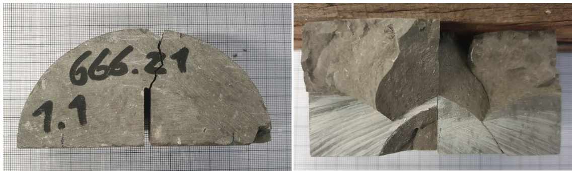
Fig. 5-1: Example of test specimen after testing The crack does not follow a parallel plane to the notch.
