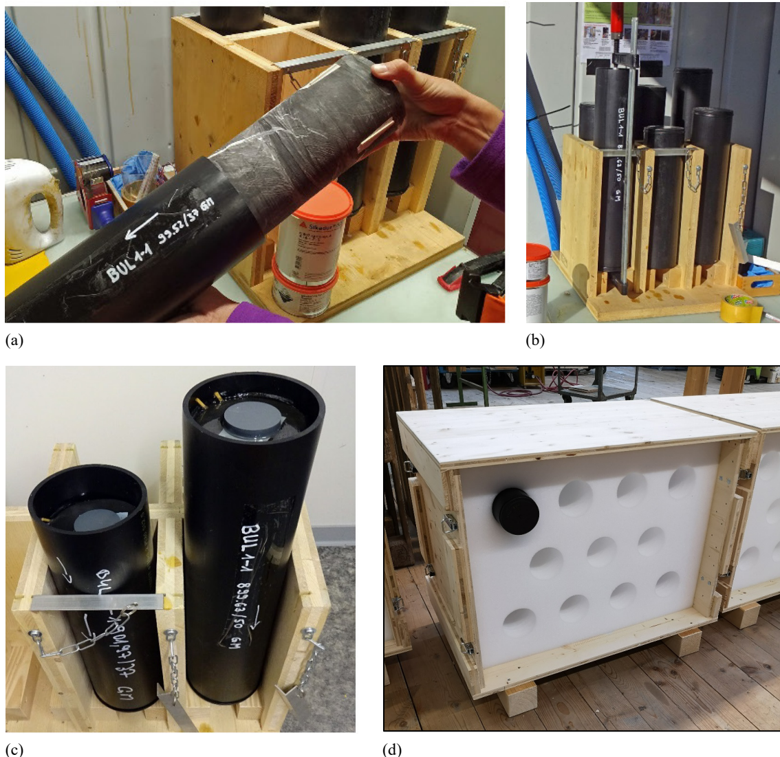
Fig. 3-1: Sampling and storage workflow of GM cores
