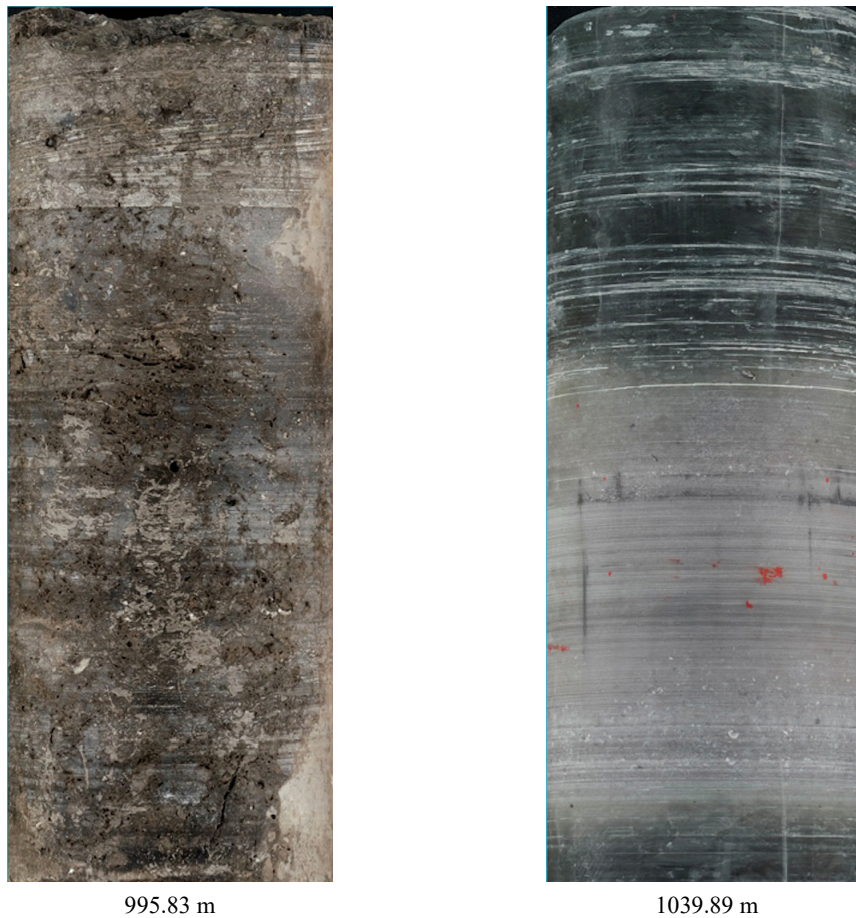
Fig. 4.3-3: Core photographs of heterogeneous samples from the Keuper Width of photographs is 10 cm.
