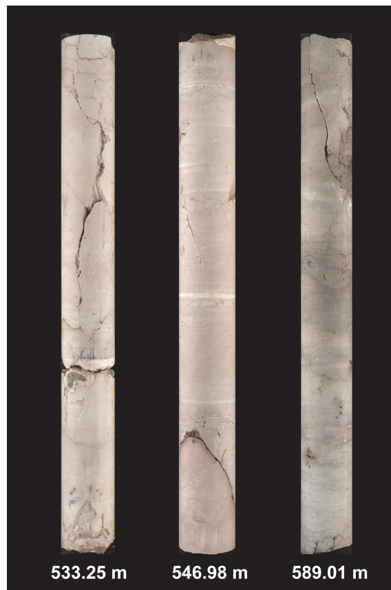
Fig. 5.8-1: Core photographs of fractures in the «Felsenkalke» + «Massenkalk» Width of drill core is 10 cm.
