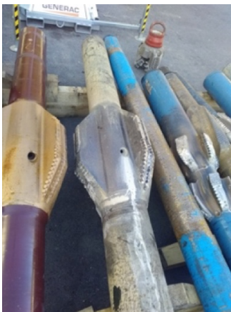
Fig. H-24: Bit #19, 17½" hole opener, drilled from 498.00 m to 710.65 m MD
