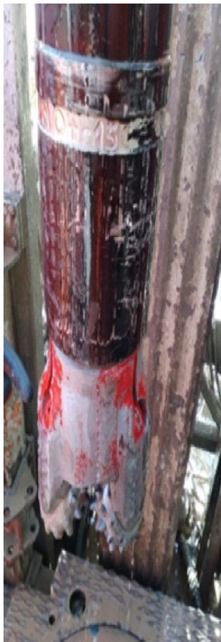
Fig. H-30: Bit #47, BHA #62 (stabiliser with OD larger than 6%", hanging up)
