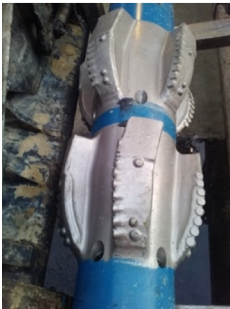
Fig. H-23: Bit #18, 12¼" hole opener, drilled from 505 m to 710.70 m MD
