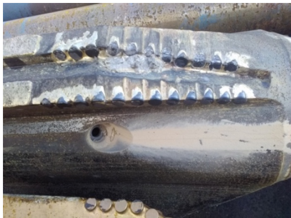
Fig. H-24: Bit #19, 17½" hole opener, drilled from 498.00 m to 710.65 m MD
