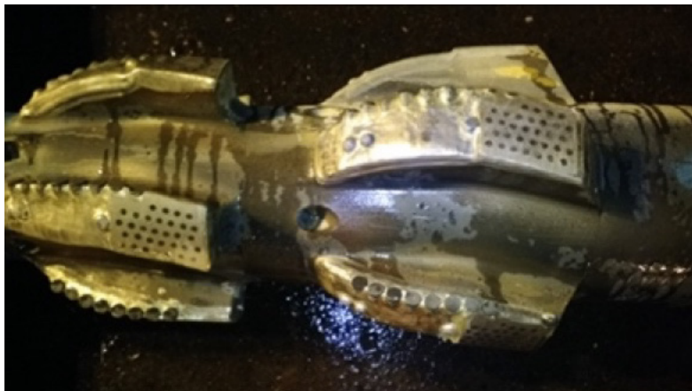
Fig. H-23: Bit #18, 12¼" hole opener, drilled from 505 m to 710.70 m MD
