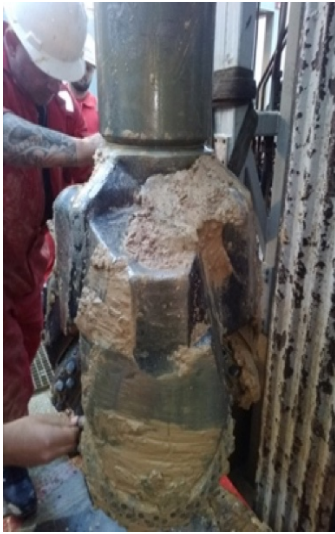
Fig. H-15: Bit #1, drilled from 40 m to 229 m MD, balled up with clay
