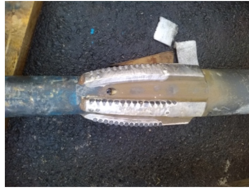
Fig. H-22: Bit #17, 8½" hole opener, drilled from 505 m to 711.80 m MD
