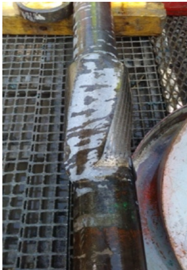
Fig. H-30: Bit #47, BHA #62 (stabiliser with OD larger than 6%", hanging up)
