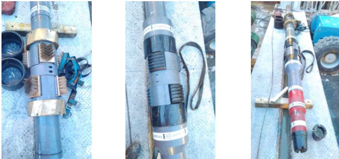
Fig. H-27: Bottom hole assembly (BHA) #38, scraper run with 8 \frac{3}{8} " bit
