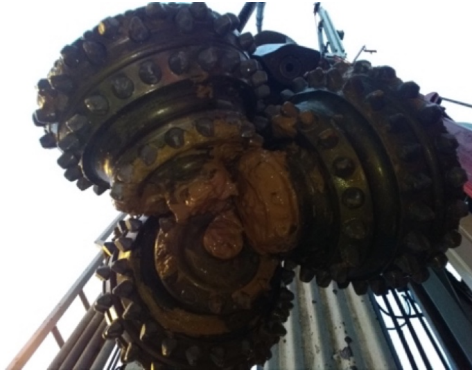
Fig. H-15: Bit #1, drilled from 40 m to 229 m MD, balled up with clay
