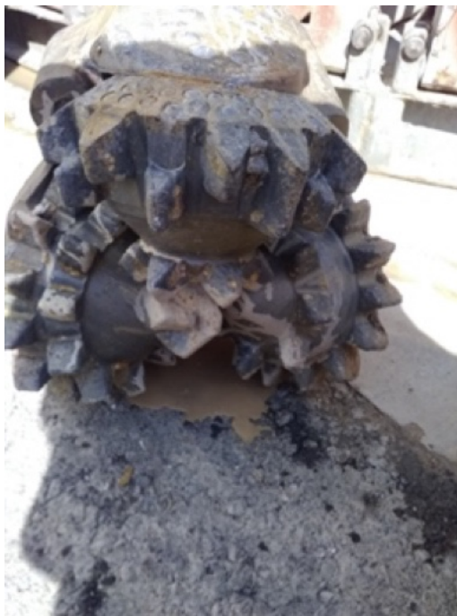
Fig. H-18: Bit #5, drilled from 479 m to 498 m MD
