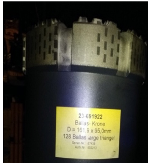
Fig. H-19: Core Bit #6, run in hole (RIH), drilled from 498 m to 505.18 m MD
