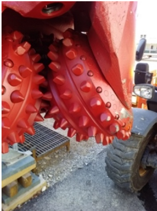
Fig. H-17: Bit #3, drilled from 323.4 m to 493 m MD
