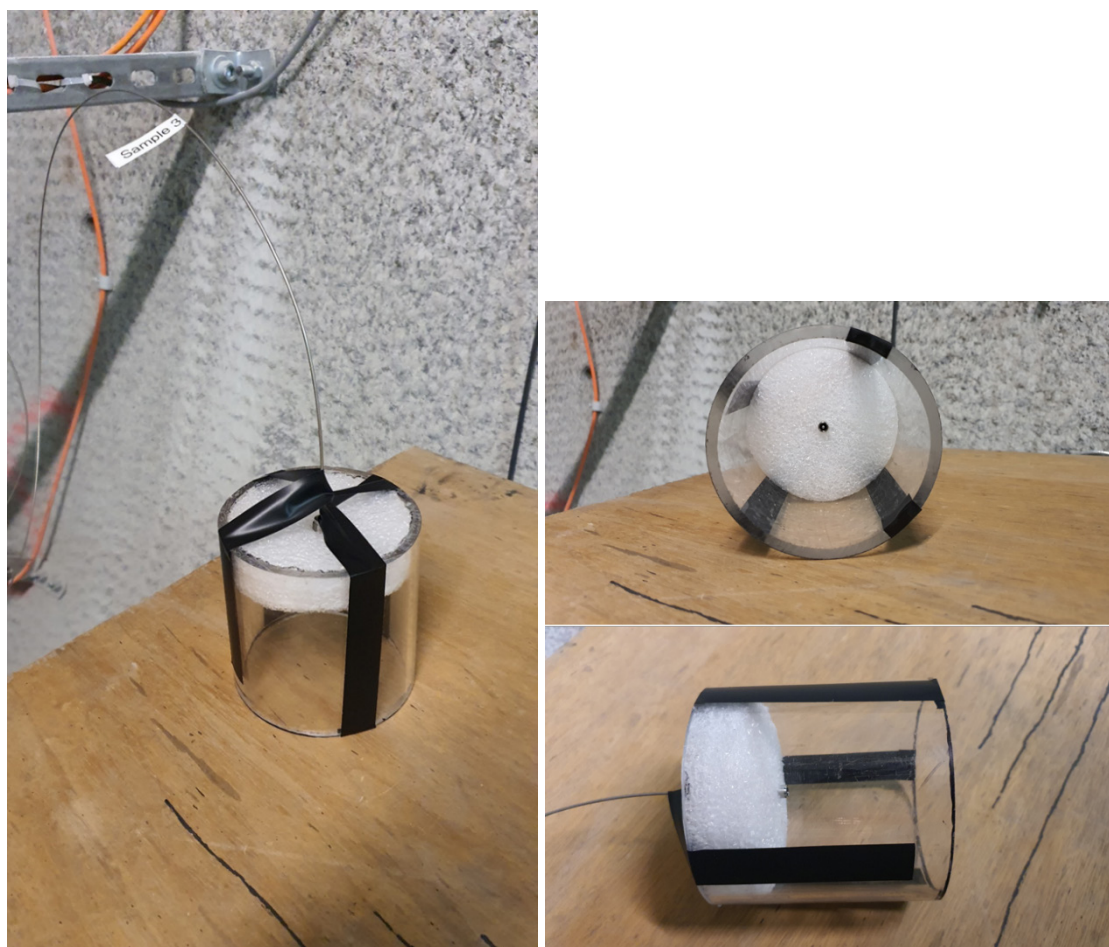
Fig. 3-8: Protector holding the third sniffing capillary for flexible deployment at different positions at the GAST plug and its vicinity
