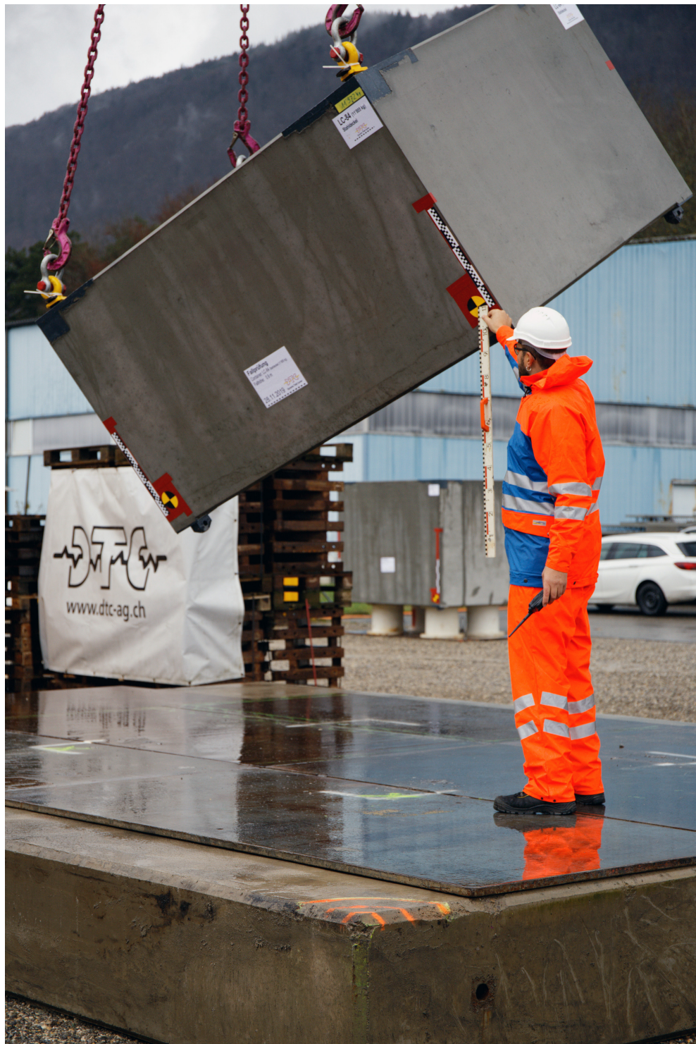
Fig. 8-12: Preparation of LC-84 for a Type A package drop test
