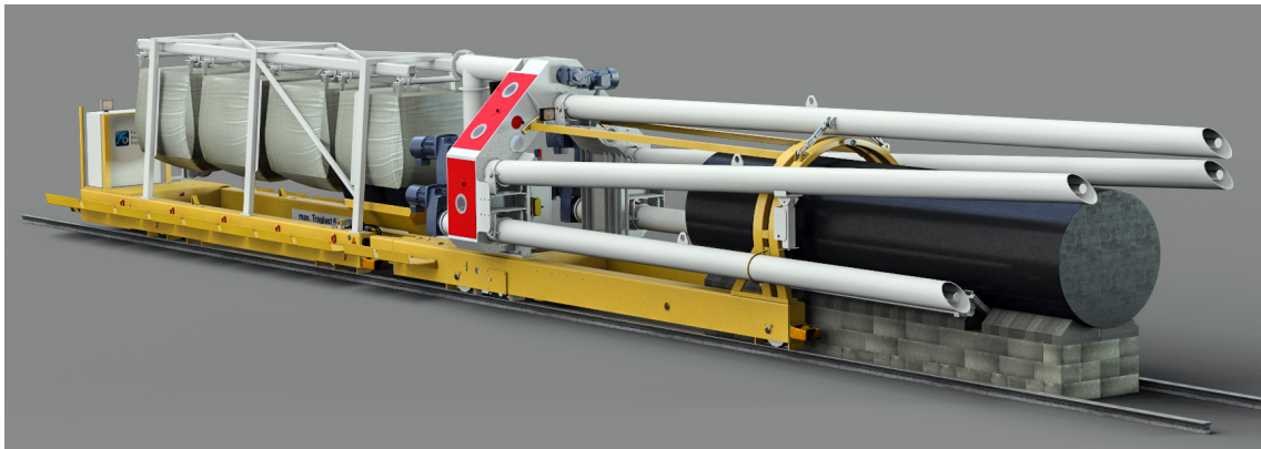
Fig. 8-9: Illustration of the 17-metre-long buffer emplacement machine built for the FE experiment
