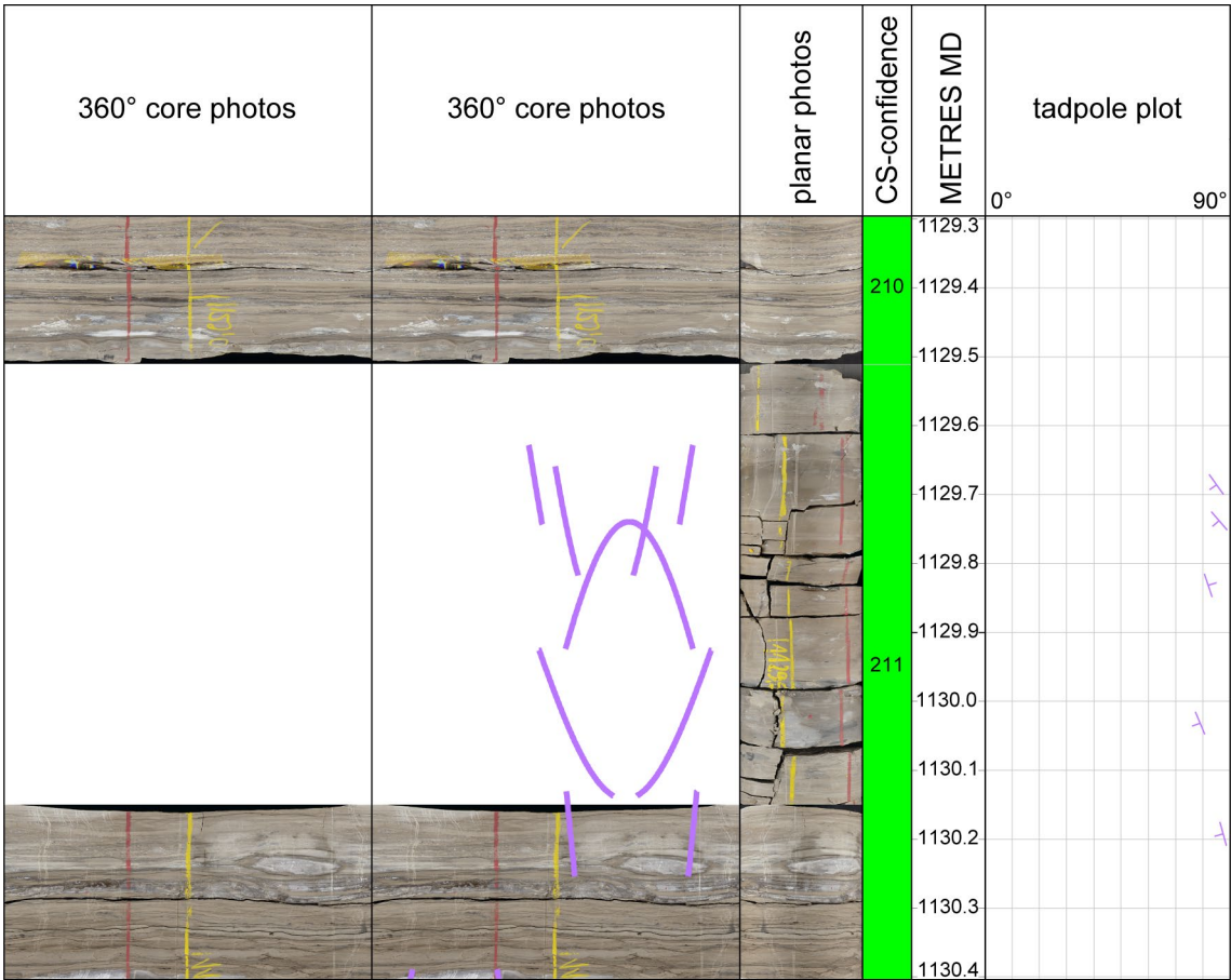
Fig. 2-5: Interval without 360° core photographs from 1'129.50 m to 1'130.15 m MD (log depth) in the Zeglingen Formation In this example, the core goniometry and structural analysis were performed on the drill core. The orientation data were determined with a geological compass and subsequently imported into the digital dip database of TerraStation II. The goniometry confidence for this core section is high (column "CS-confidence", green).
