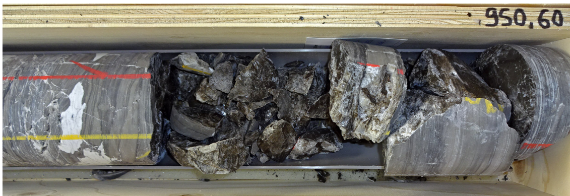
Fig. 3-10: Fault zone with FDC 2
