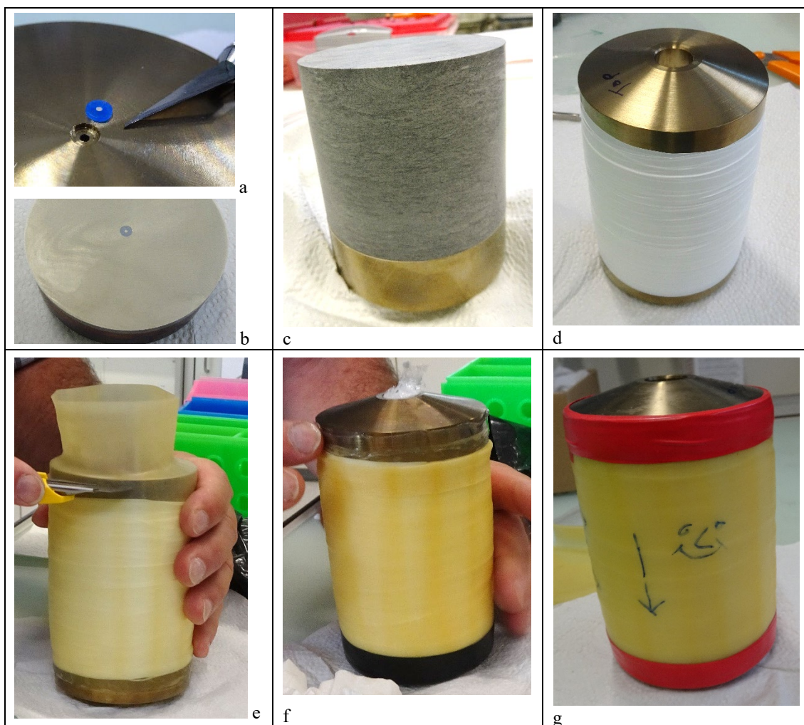
Fig. 9-5: Preparation of core assembly for advective displacement.
