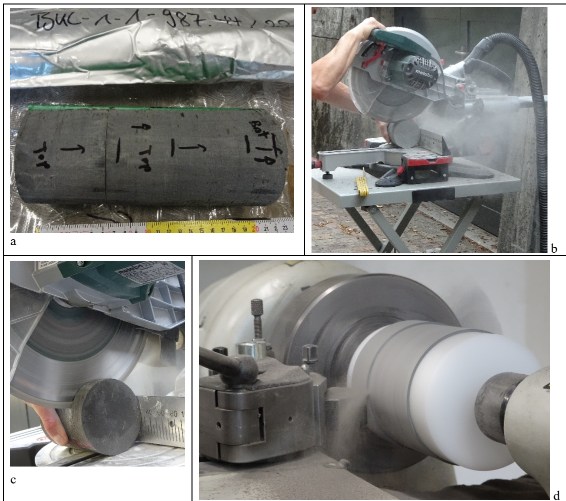
Fig. 9-4: Initial steps of sample inspection, cutting and turning.
