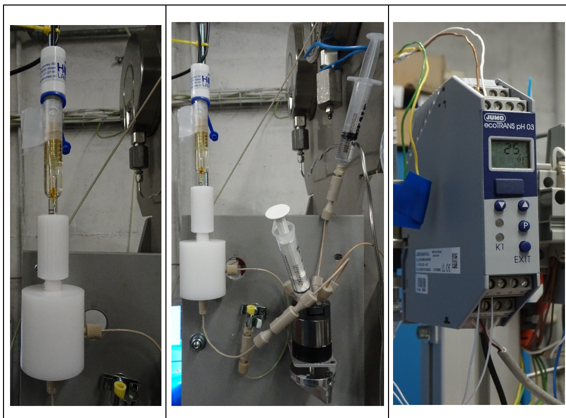
Fig. 9-8: Minitaure pH flow-through cell with micro Ross electrode.
