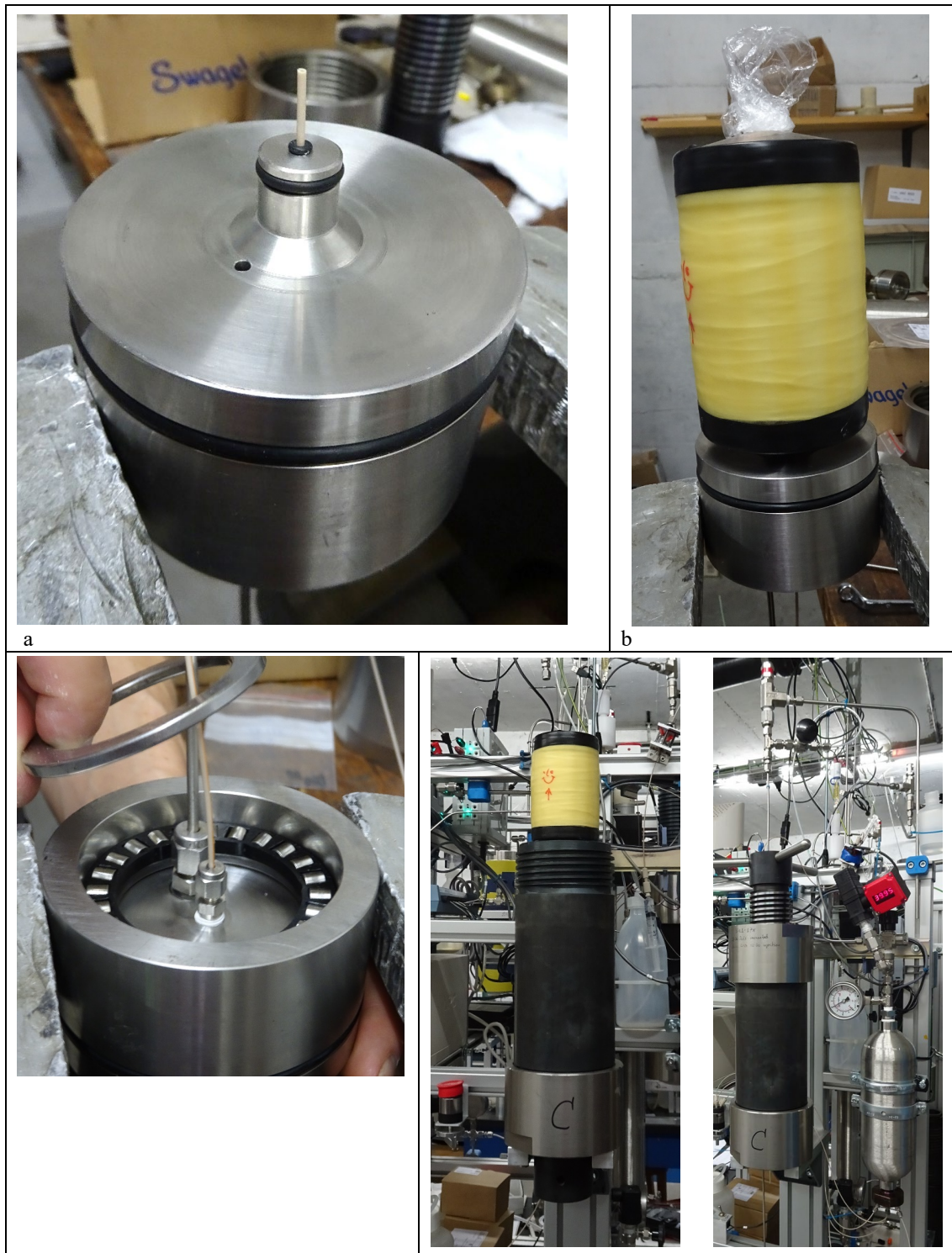
Fig. 9-6: Mounting of a core assembly (core sample, DM 80 mm, with titanium end pieces) into a pressure vessel for an advective displacement experiment (see text for details).
