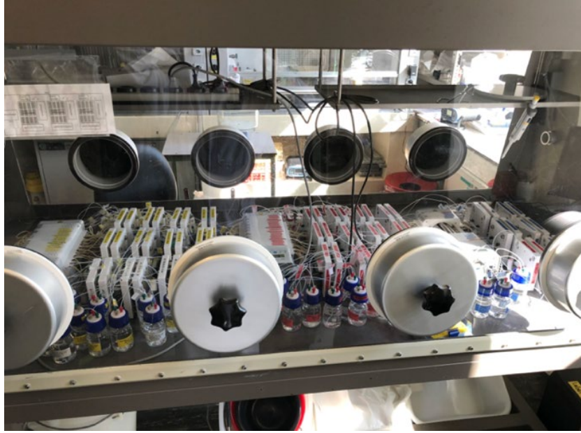
Fig. 2-5: MBraun glovebox (N 2 /CO 2 ) with diffusion cells
