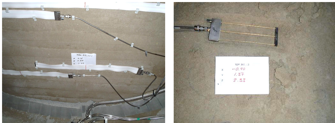
Fig. F-1: TDR sensors. Left) TDLs at S13, right) TDP
