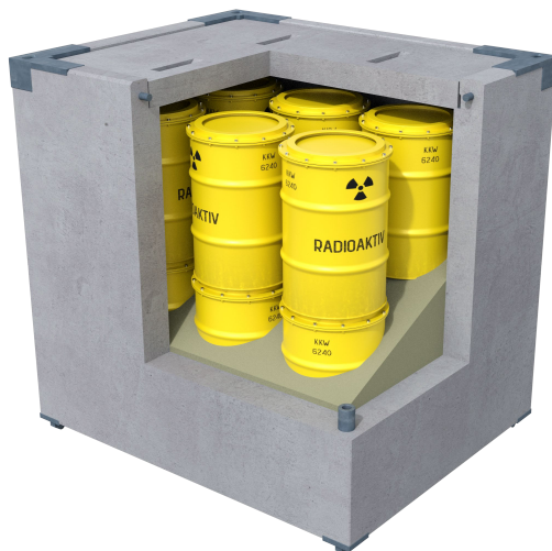
Fig. 2-12: Representation of a disposal container filled with 200 L steel drums containing L/ILW (waste packages) and backfilled with mortar
