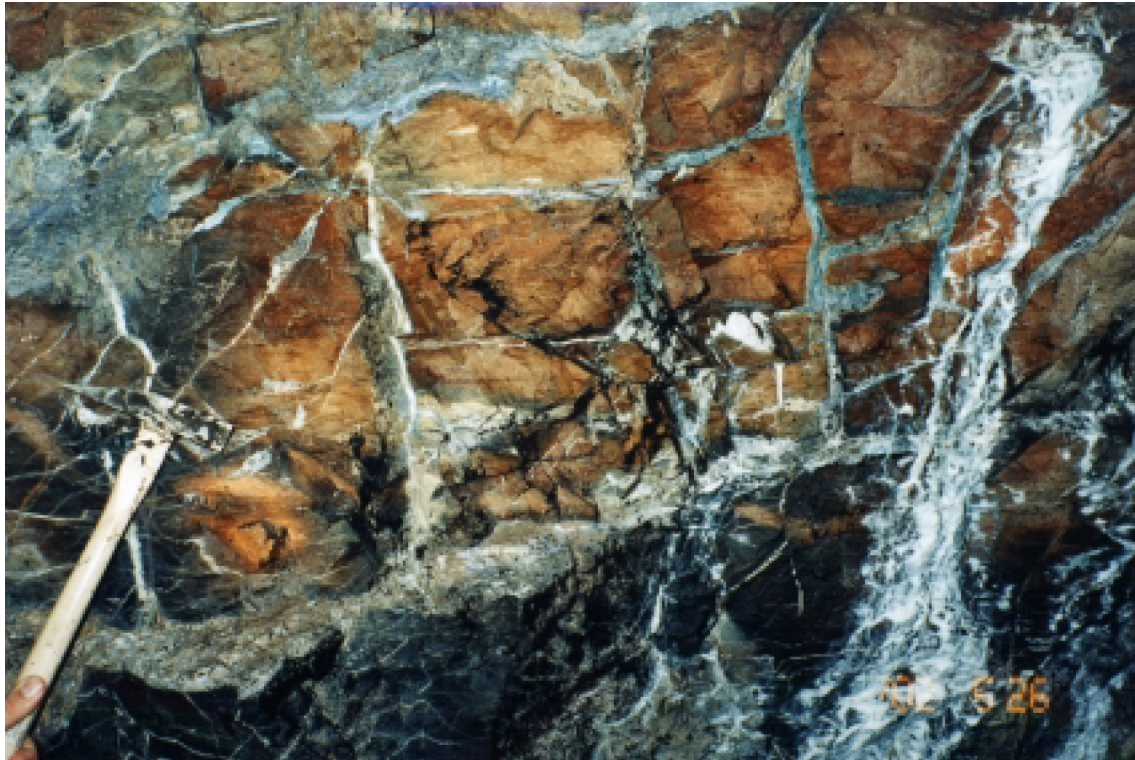
Fig. 9-2: Heavily fractured micrite host rock with abundant sealed fractures containing a comparable product to natural concretes at the Maqarin site in Jordan
