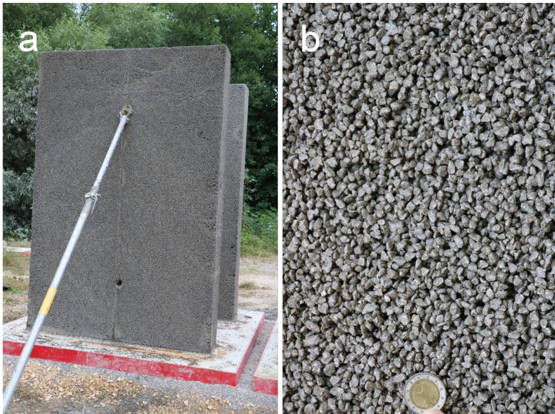
Fig. 6-6: Grain-supported cavern backfill mortar for the L/ILW caverns
