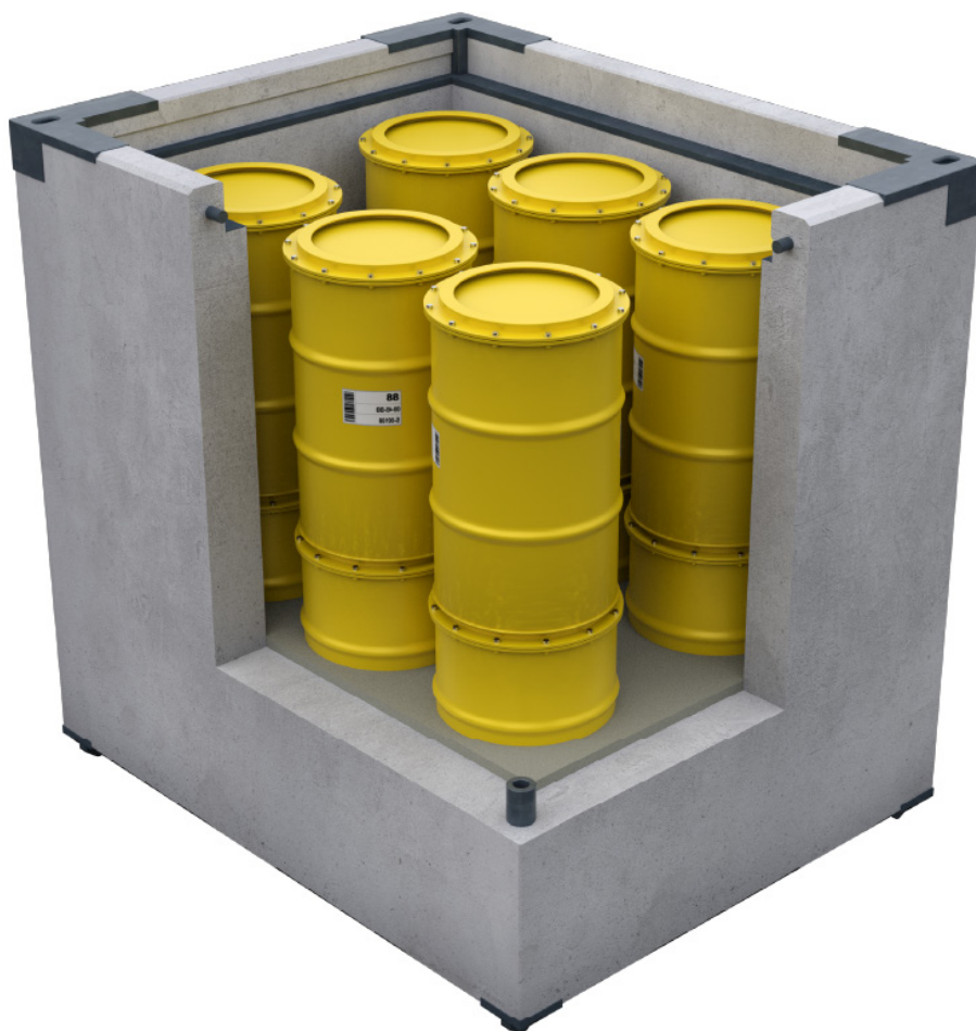
Fig. 2-5: L/ILW disposal containers (LC) filled with waste drums
