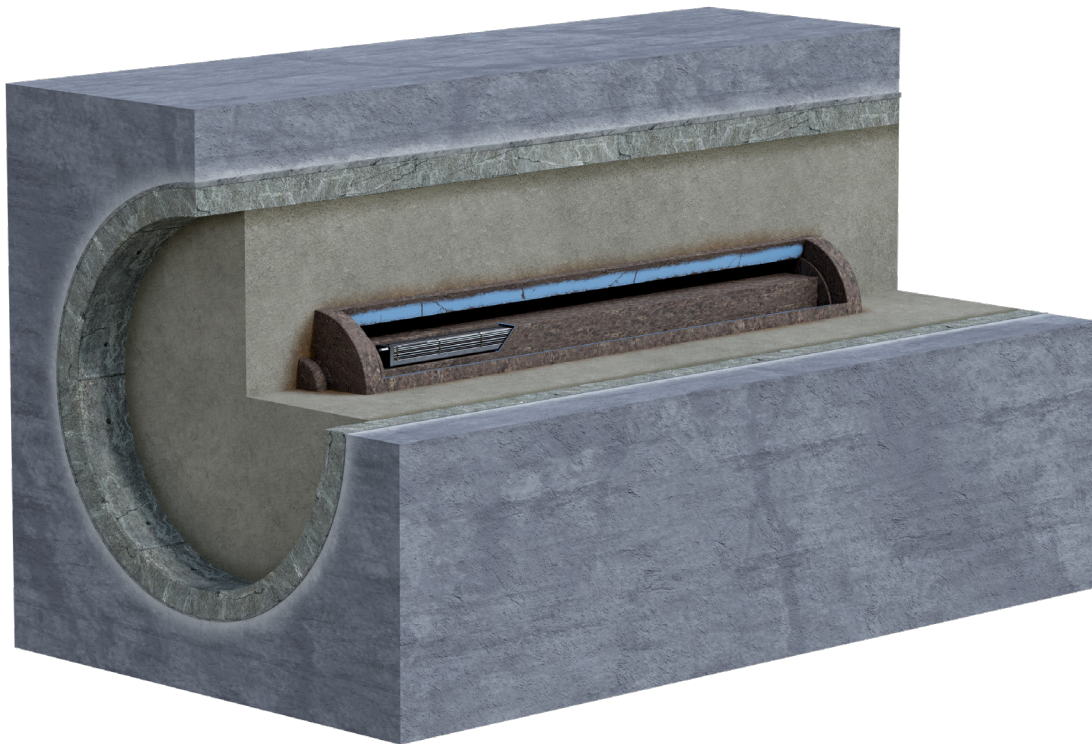
Fig. 7-3: An illustrative representation of an HLW emplacement drift in the period following deep geological repository closure
