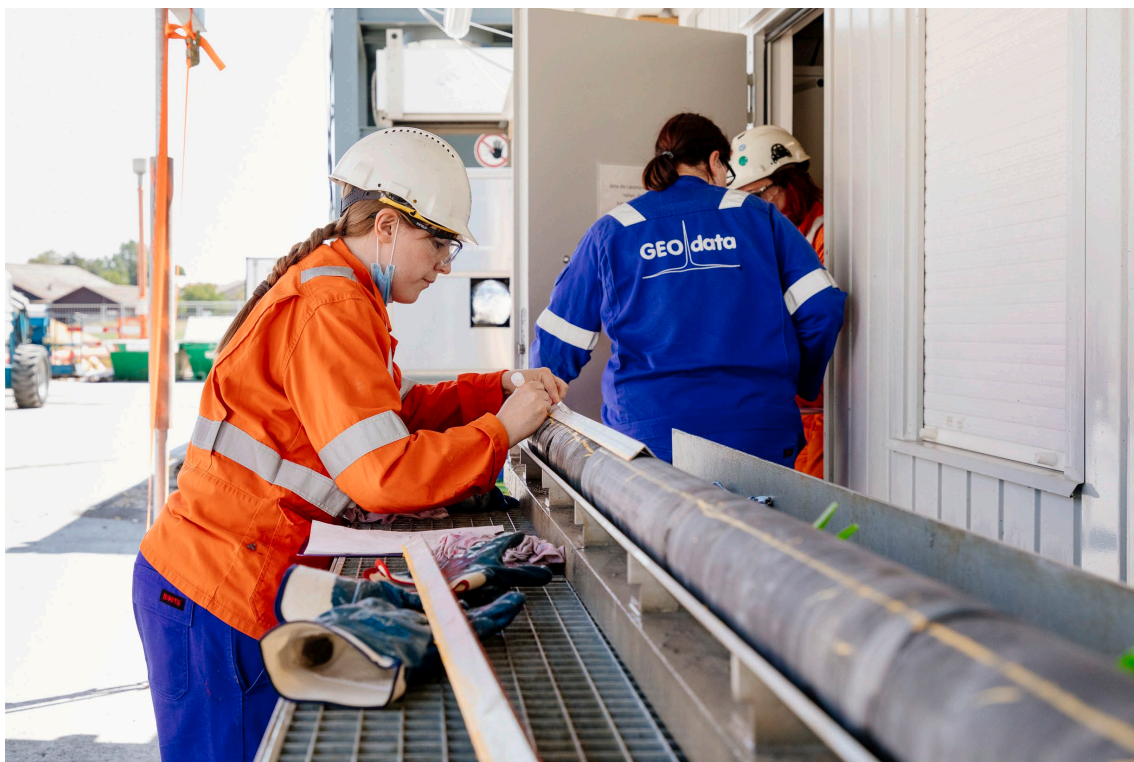
Fig. 2-5: A core is marked with orientation lines
