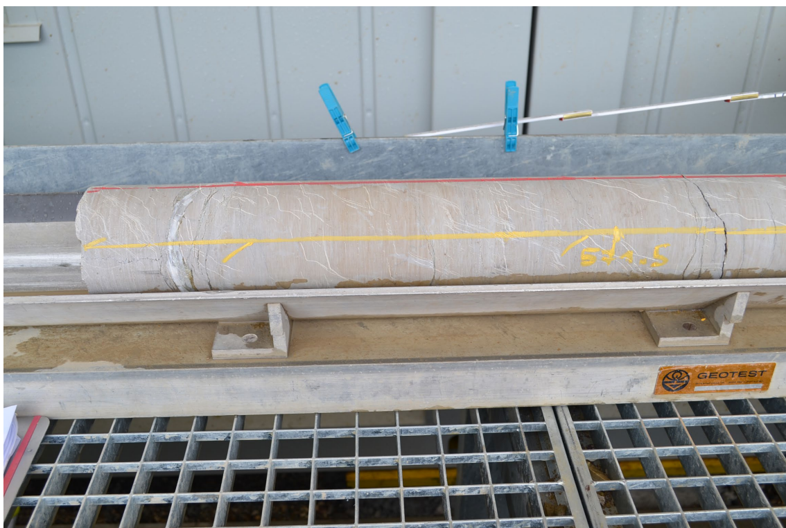
Fig. 2-6: Cleaned, measured and marked core
