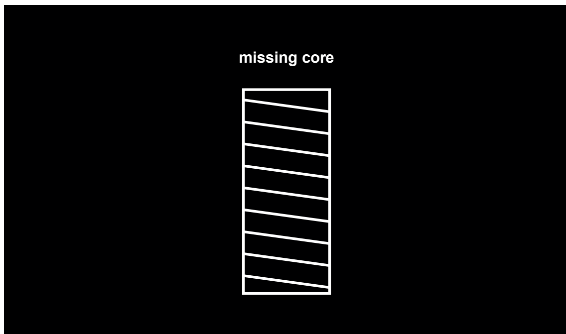
Fig. 2-10: White hachures signature used for missing core due to FIT pilot hole or drilling related technical issues in the composite displays
