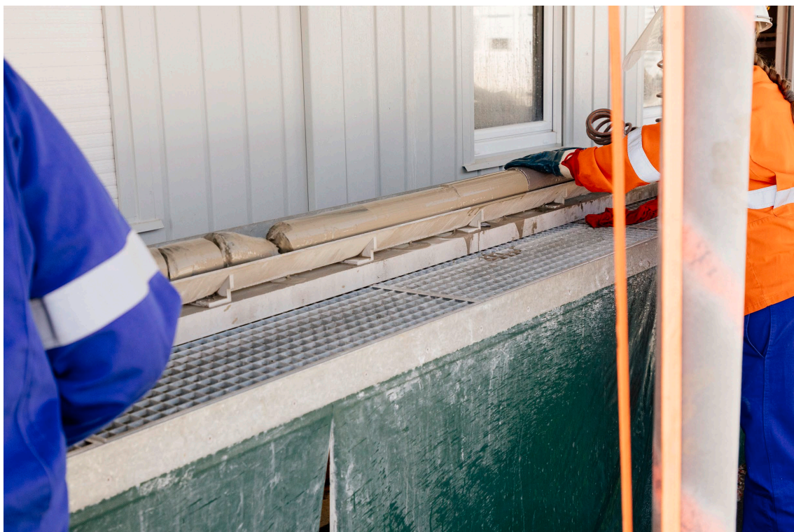
Fig. 2-3: A core covered in drilling fluid on the core processing table
