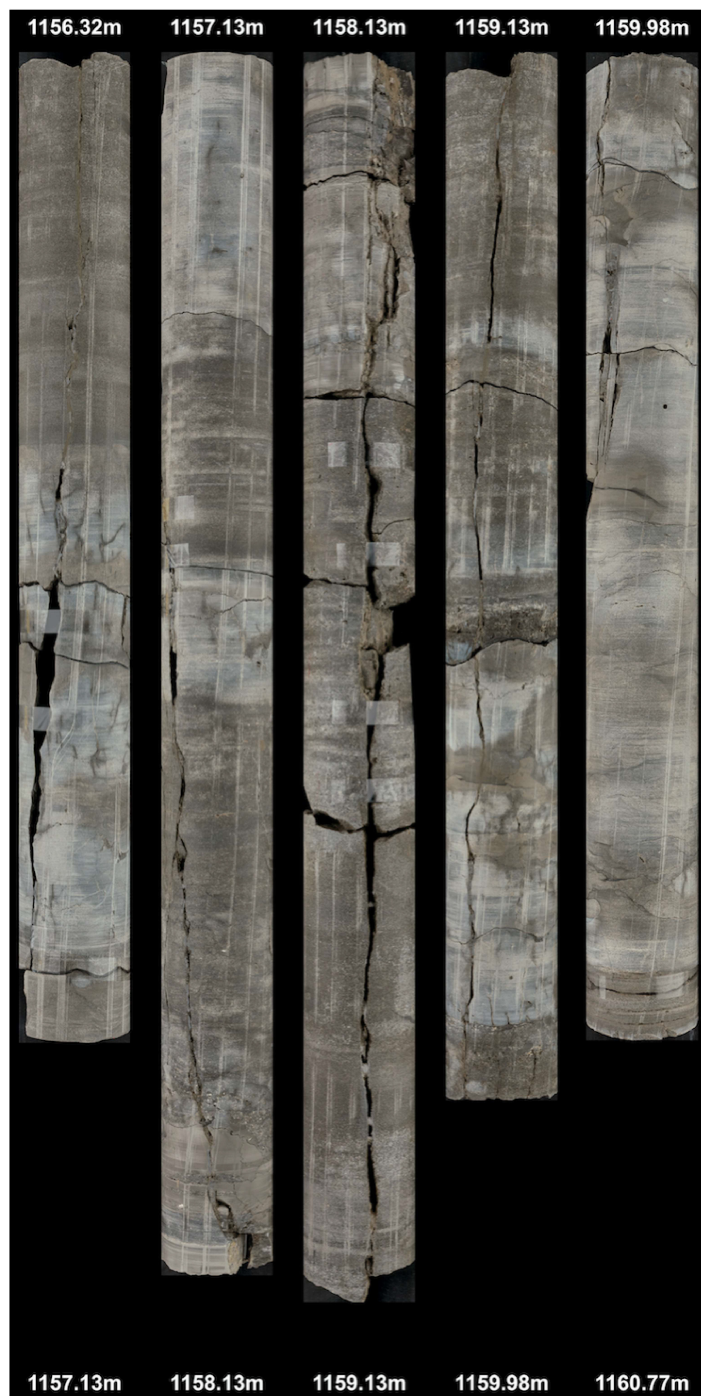
Fig. 5.4-1: Vertical joint in the dolomites of the Stamberg Member (Schinznach Formation) Core diameter is 10 cm.
